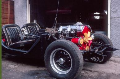
Attention was then turned to the body shell, stripped to bare metal, new wings and sills. Apart from the wings and sills, it proved to be in reasonable condition.
