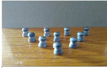
Photo5; The lead pellets. These are domed for target practice rather than pointed for hunting.
