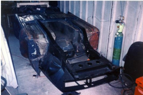
New front end fitted
