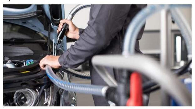
To ensure the optimum performance of your Land Rover, it is important to keep your Diesel Exhaust Fluid – also known as AdBlue – topped up. The fluid is essential for neutralising harmful gases generated in the engine and helps to reduce the emissions from the exhaust by up to 90%.
