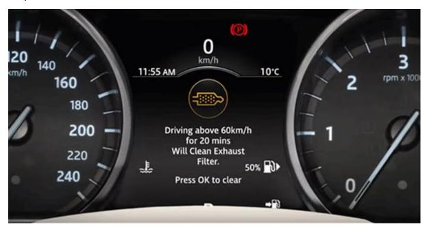
Since 2009, all Land Rover diesel vehicles have been fitted with a Diesel Particulate Filter. This important device captures 99% of soot and particulates from the engine to help significantly reduce emissions. It is essential that to prevent the particulates from building up in the filter, and to avoid any impact to the performance of your vehicle, that this soot is 'burned off' through a process called regeneration.
